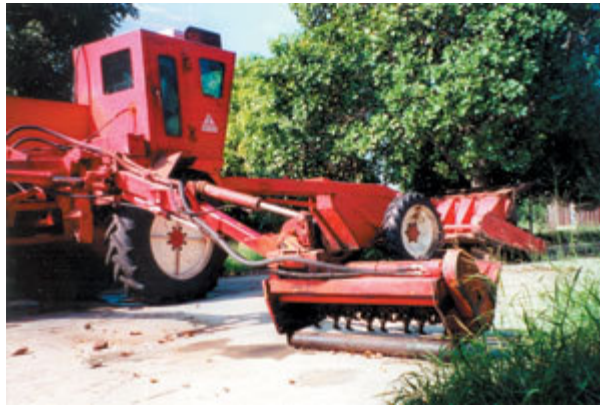
Agri-flail machines, modified agricultural tractor frames, were developed to absorb explosions of mines planted .8 of an inch underground. The use of these new machines, in addition to the arrival of the dog teams, has more than doubled the rate of cleared lands in Mozambique in the last year. Image by:Paul Dirdak, UMCOR Source: New World Outlook
